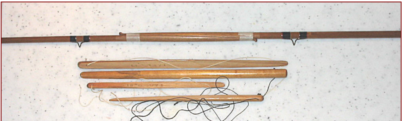
Fig. 14a + b: “Grant Vibration”, bottom and top splices joined with tape. The severe swell over the splices is clearly visible, (cf. Fig. 8). Also pictured the splice protectors, with rod length and number stamped into the flats.
